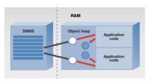
Being memory centric open up opportunities in communication between the application and data. Starcounter has a patented innovation called VMDBMS. In traditional databases, the data and the application are stored in different parts of the RAM. In Starcounter we have integrated the application with the DBMS, making it possible for both the application and the DBMS to share the objects. With this patented innovation, there is no need to move data between different places in
